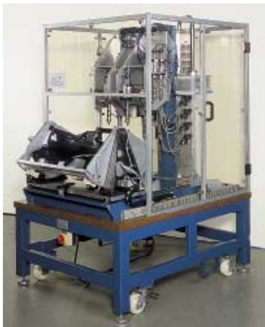
10-item thermal installation (HES) semi-automatic
