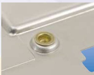
Rivet couplings, M 1.6 with increased torsional strength for shield plates (0.3 mm thickness of material)
