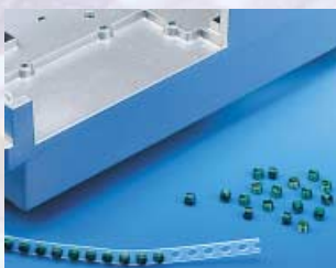
Mounting plate for telecommunications base stations, magnesium precision casting, HELICOIL® plus Threaded inserts M 3 made of aluminum alloy, artificial ageing, hard coating, coated with lubricant. Material: Al Zn Mg Cu 1.5
